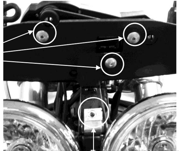
Location of the bracket and the threaded fastener
